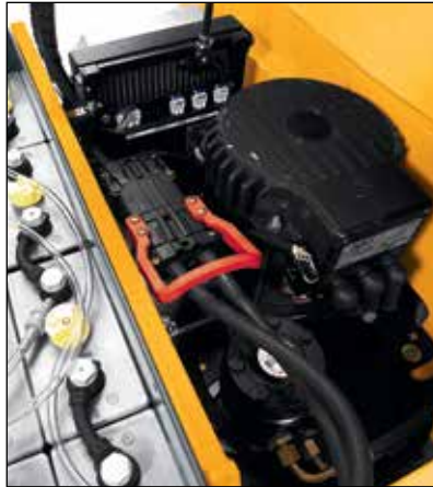
Drive and lift motor with AC technology
