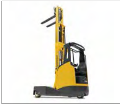
Jungheinrich mast design reduces sway at high lift heights.
