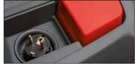
Easy-to-operate main connector for on-board charger
